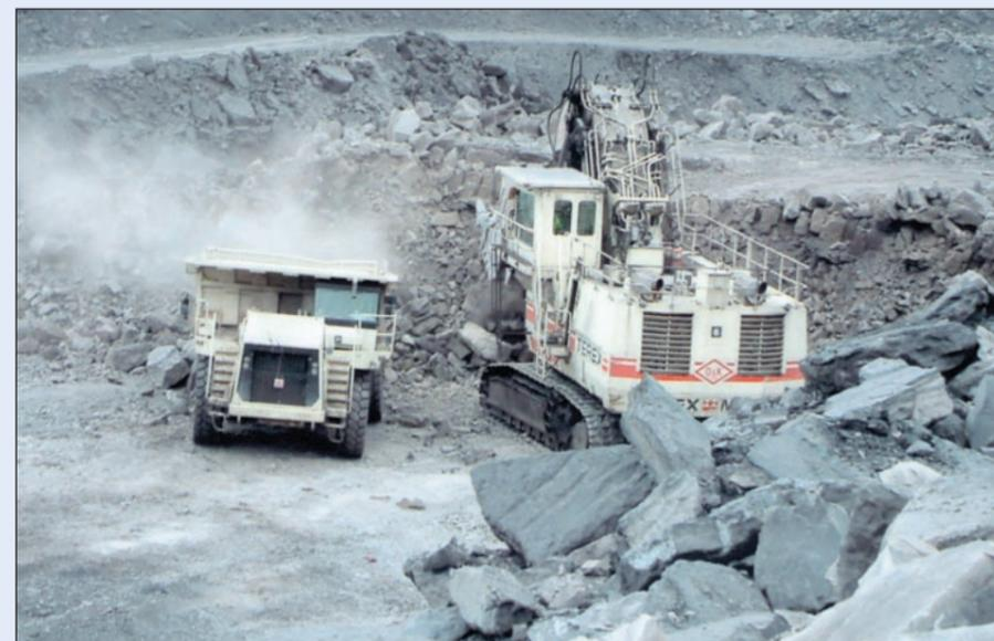
An excavator loads a 100-tonne-capacity dump truck at the Garleffan opencast site.
