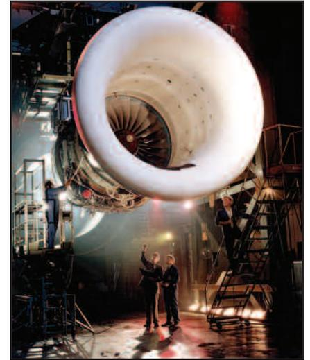
Trent 700 engine test. Voyager is powered by Rolls Royce Trent 772B – 71,000 lbf
