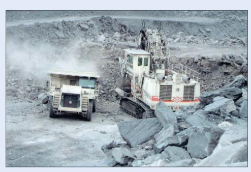
An excavator loads a 100-tonne-capacity dump truck at the Garleffan opencast site.
