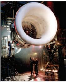
Trent 700 engine test. Voyager is powered by Rolls Royce Trent 772B - 71,000 lbf
