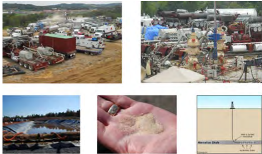
Figure 3: A busy drill pad with frac fleet. A well is hydraulically fractured in multiple stages. Typically 450 tonnes of sand (or bauxite) per well are used to prop the water-pressure-induced fractures. Source: Photos by Doug Duncan, USGS. Marcellus Shale gas play of southwestern Pennsylvania.
