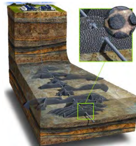
Figure 4: Hydraulic Fracturing in the Oil & Gas Industry: Source Schlumberger ‘hiway’ technology (also: Liberty, Halliburton, Baker-Hughes etc).
